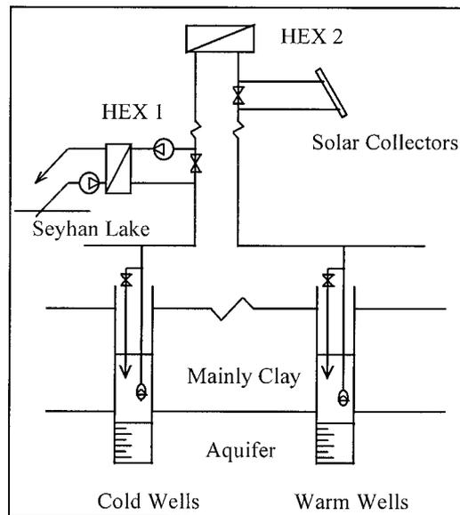
Fig. 2. Layout of the ATEs system with solar collectors.
