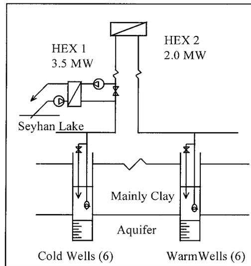
Fig. 1. Layout of the ATEs system.
